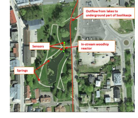
Channel dimensions: 14,6 x 3 m Water level: 0,66 ... 1,05 m Sediment layer: 0,2...0,4 m Wood chips placed: 7,5 m<sup>3</sup> Q = 1,6 ... 2,5 l/s
